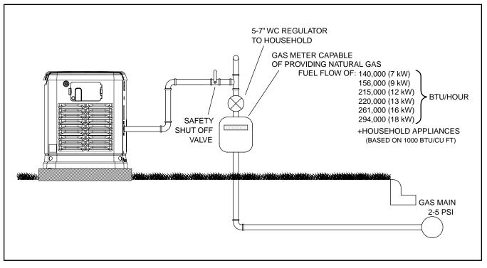
Figure 2. Proper Fuel Installation
